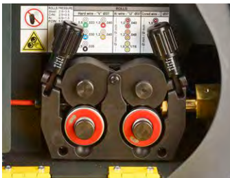
Professional double groove feeding mechanism with 4 rolls
